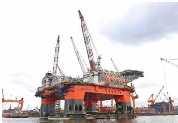
Safe Zephyrus is the second accommodation semi-submersible unit Sembcorp Marine has built for Prosafe
