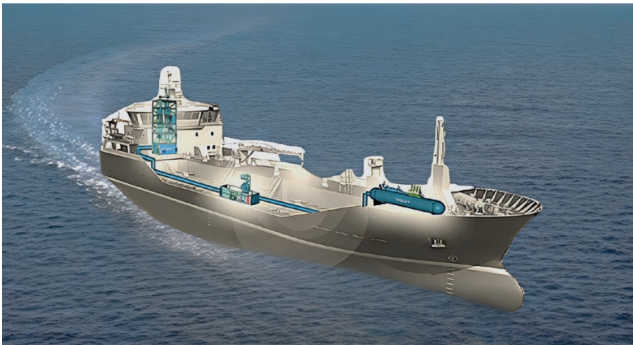
The innovative SEARA™ Onboard Carbon Capture System, jointly developed by Aragon and Seatrium Eco Technology, integrates efficient CO 2 capture, liquefaction, purification, and storage technologies into a single compact solution
