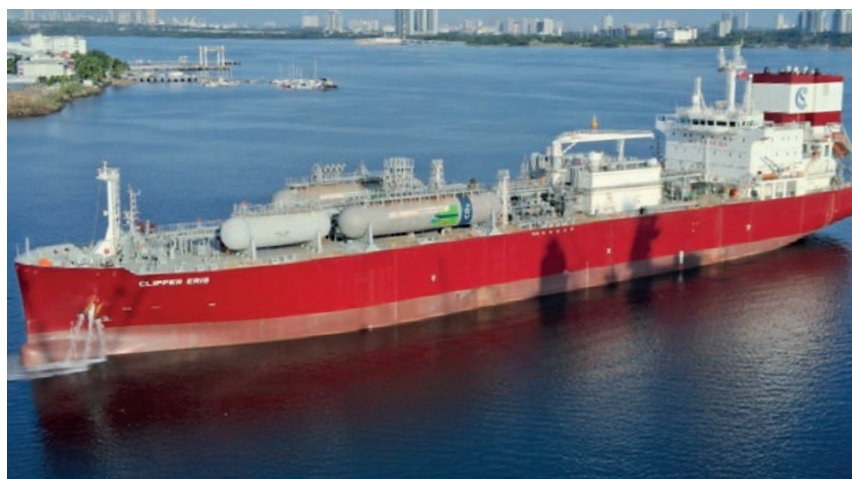
Seatrium completed the world's first full-scale, turnkey CCS retrofit on Solvang's ethylene carrier, Clipper Eris, which is set to capture up to 70% of CO 2 emissions using amine cleaning technology
