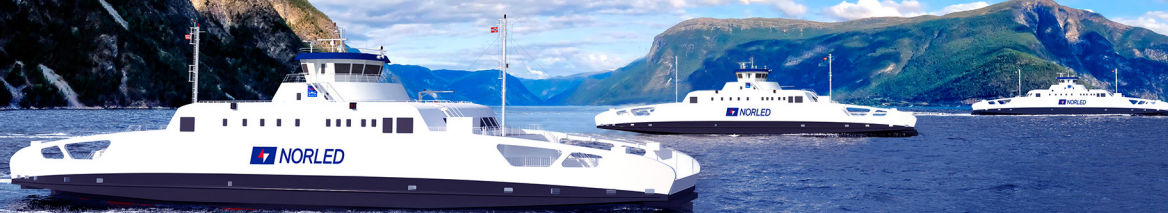
Three zero-emission fully battery-operated Roll-on/Roll-off Passenger (Ropax) Ferries designed, built and optimised by Sembcorp Marine
