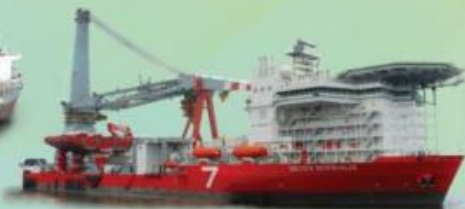
Newbuild of a self-propelled DP-3 heavy lift pipelay vessel
