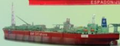
Conversion of tanker to FPSU
