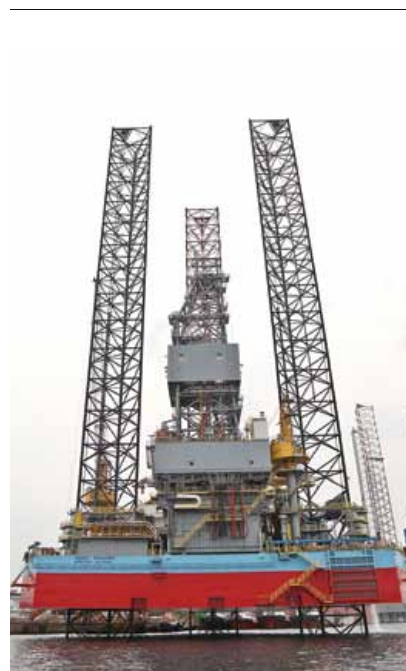
Maersk Highlander – a Friede & Goldman JU 2000E jack-up for harsh-environment operations in the UK North Sea Culzean field development
