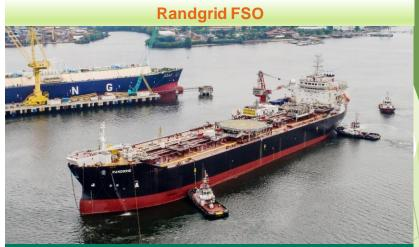
**Project:** Conversion of shuttle tanker into an FSO, including fabrication and installation of new living quarters, hull reinforcements, refurbishment of submersible turret loading (STL) compartment, installation of new helideck, offshore crane, loading hose reel package and azimuth thruster, replacement of two generators, as well as piping and cabling works.
