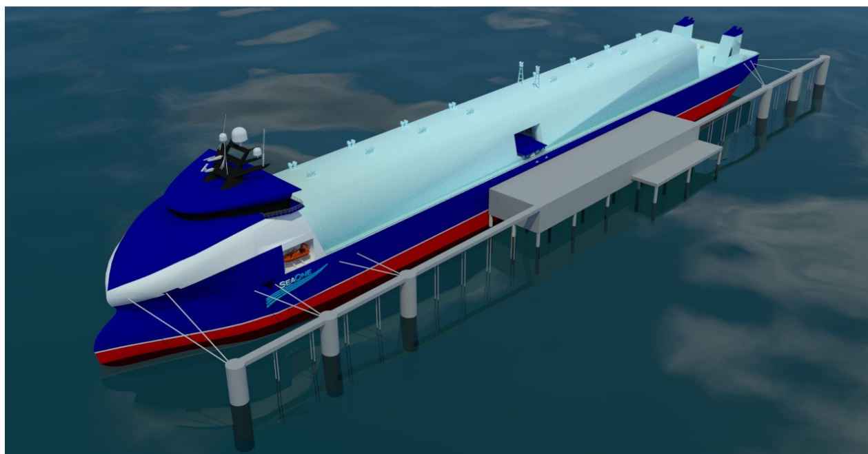
Artist's impression of the 2 Bcf capacity CGL carrier designed by Sembcorp Marine
