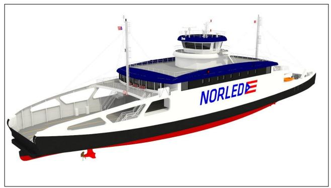
Artist's impression of the Norled hybrid plug-in ropax ferry. Three identical vessels will be completed in 4Q2020 for deployment in the Hella-Vangsnes-Dragsvik service route in Norway. During normal operations, the vessels will run on zero-emissions battery power.
