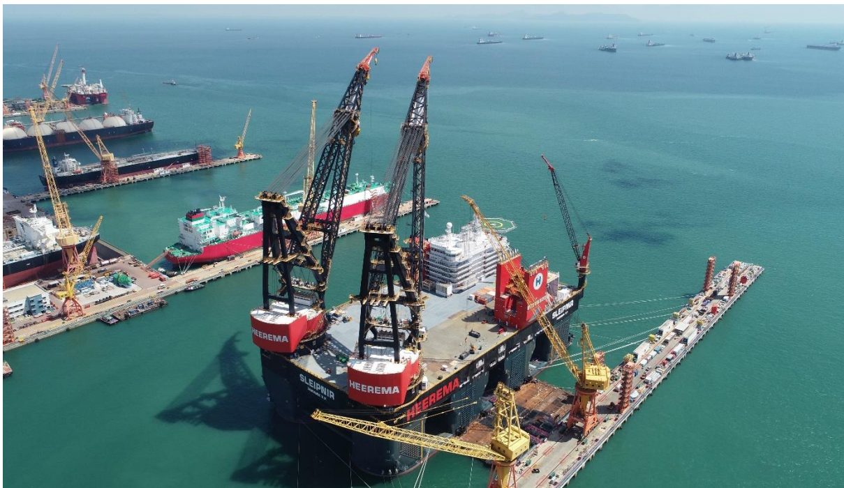
Sleipnir, the world's largest and strongest semi-submersible crane vessel built by Sembcorp Marine (b)
