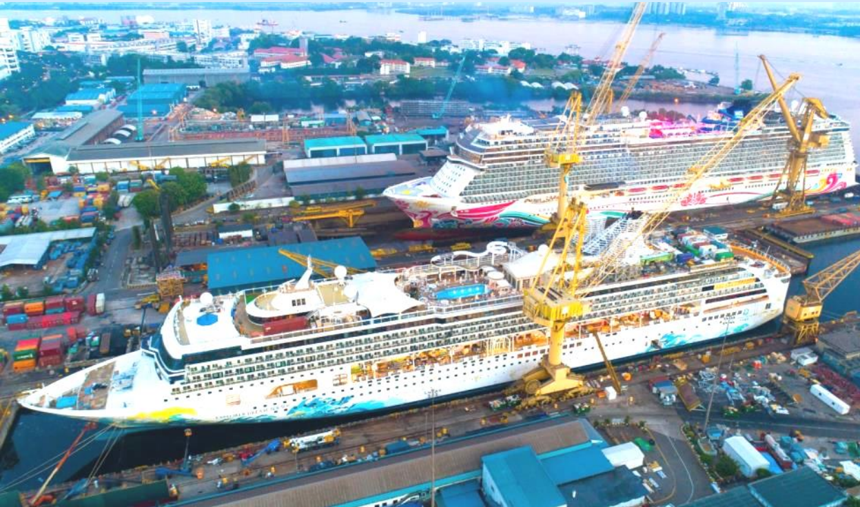
Concurrent major refit and refurbishment of Norwegian Joy for Norwegian Cruise Line and Explorer Dream (ex-SuperStar Virgo) for Genting Cruise Lines
