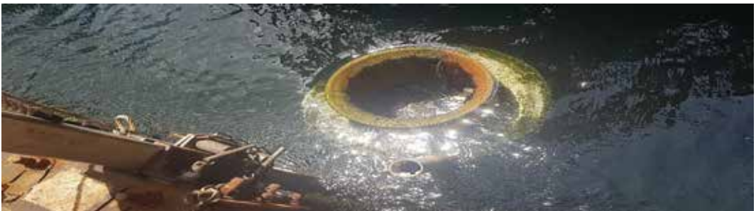
In July 2019, we installed a Seabin device (above) at our Admiralty Yard in Singapore to remove floating debris from waters around the shipyard. The collected debris and trash, such as plastic particles, pellets and wrappers, were disposed of through environmentally-responsible methods. The Seabin helped remove 240kg of floating debris in the second half of 2019.
