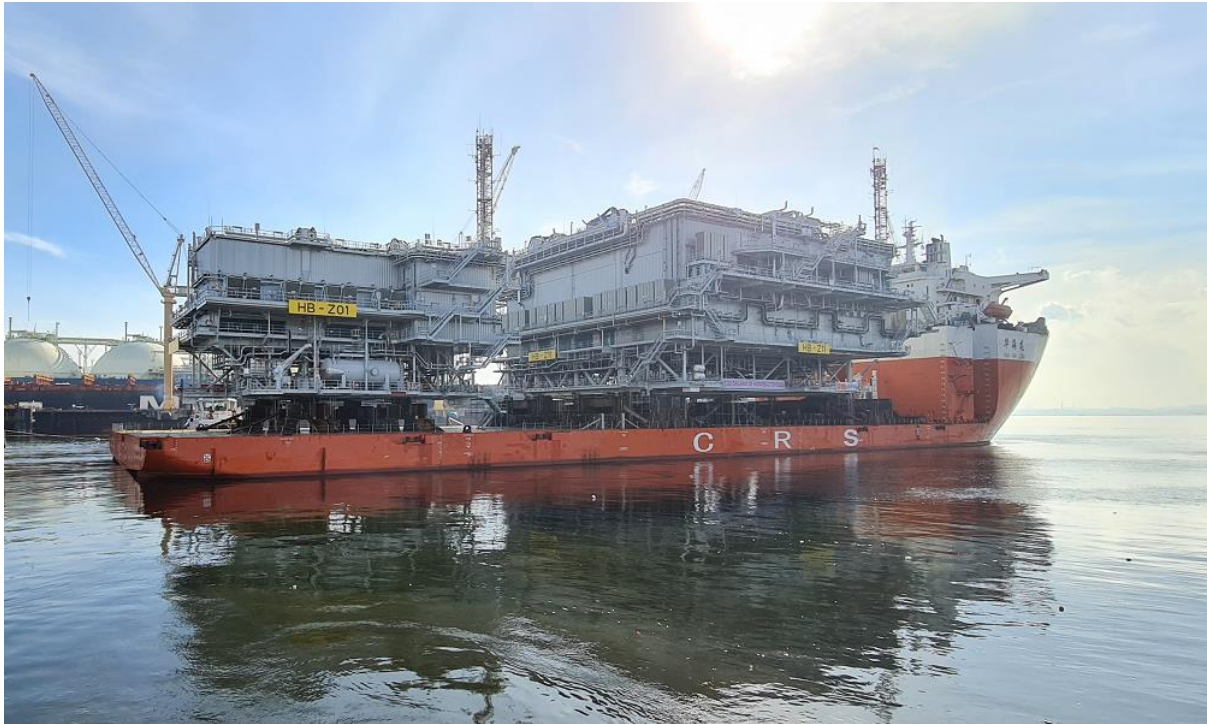
Hornsea Two's reactive compensation station and offshore substation sailing away to the UK North Sea
