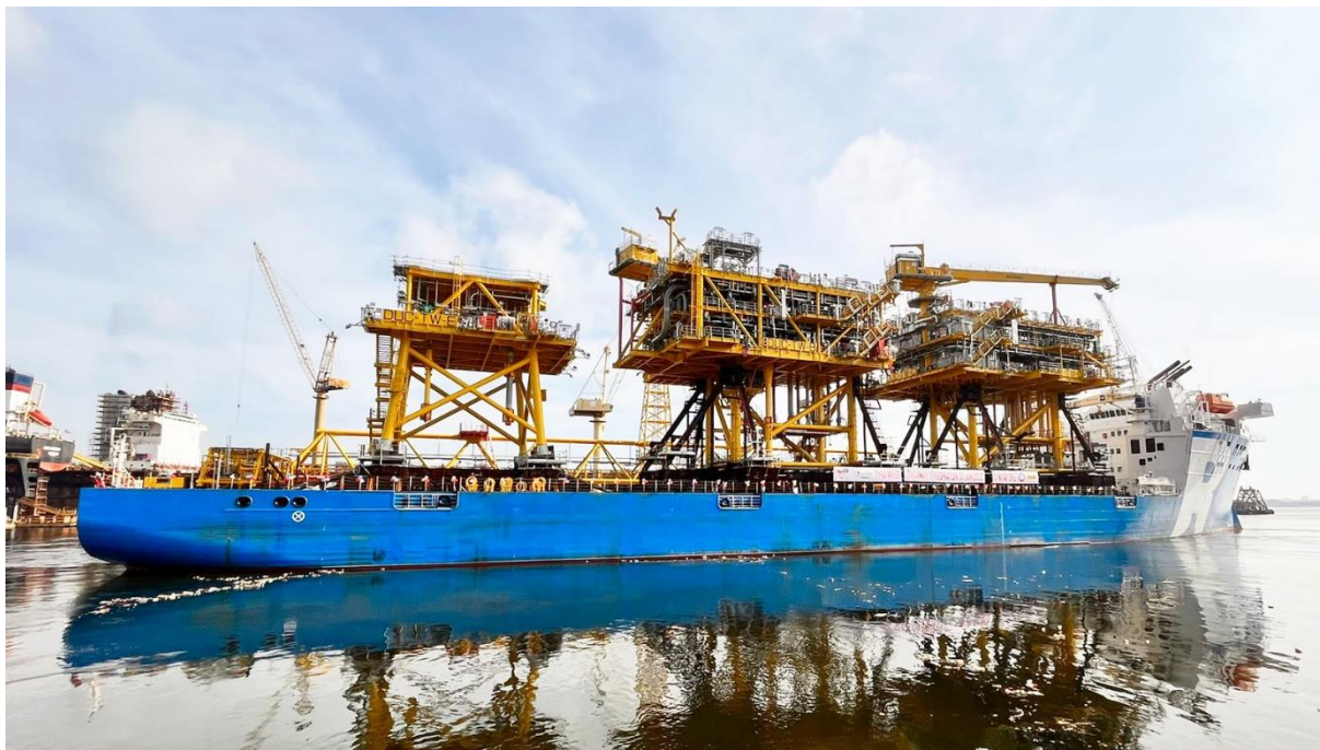
Sailaway of TotalEnergies’ topsides and bridges for Tyra West Redevelopment Field (Photo: SCM, all Rights reserved)
