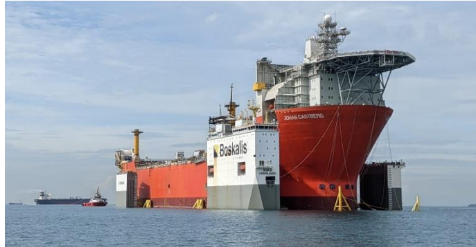
Johan Castberg FPSO transferred onto a transportation barge for its journey to Norway
