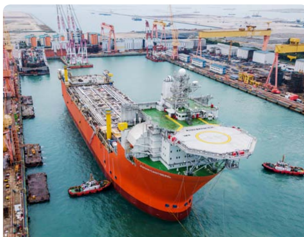
Delivered in February 2022, the Johan Castberg FPSO hull, complete with living quarters, is built to be self-contained for harsh-environment operations at the Johan Castberg Field in the Barents Sea, Norway
