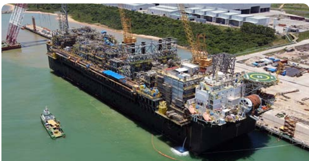
P-71 FPSO undergoing modification, integration and topside works in our Brazil yard for deployment to the Itapu Field
