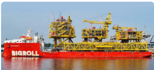
Sailaway of Tyra East production topsides and bridges
