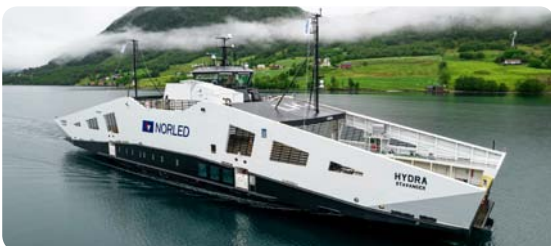
MF Hydra, the world's first liquid hydrogen-powered vessel, is a sustainable and innovative ferry designed by Sembcorp Marine's subsidiary LMG Marin
