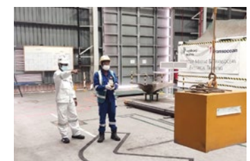
Performing overhead gantry Crane remote control operation
