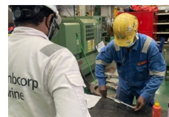
Performing portable machine drilling and tapping
