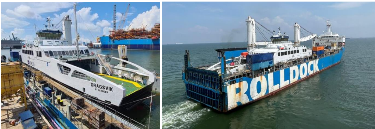
The second Ropax ferry is loaded on board dry tow transport for the sailaway to Norway ( Photos: SCM, all Rights reserved )
