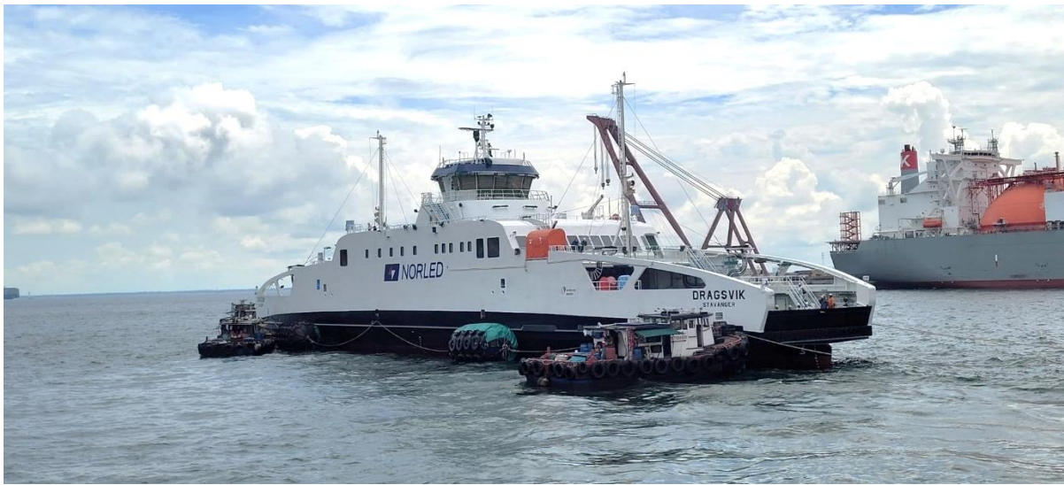
The second zero-emission battery-powered Ropax ferry designed and built by Sembcorp Marine for Norled ( Photo: SCM, all Rights reserved )
