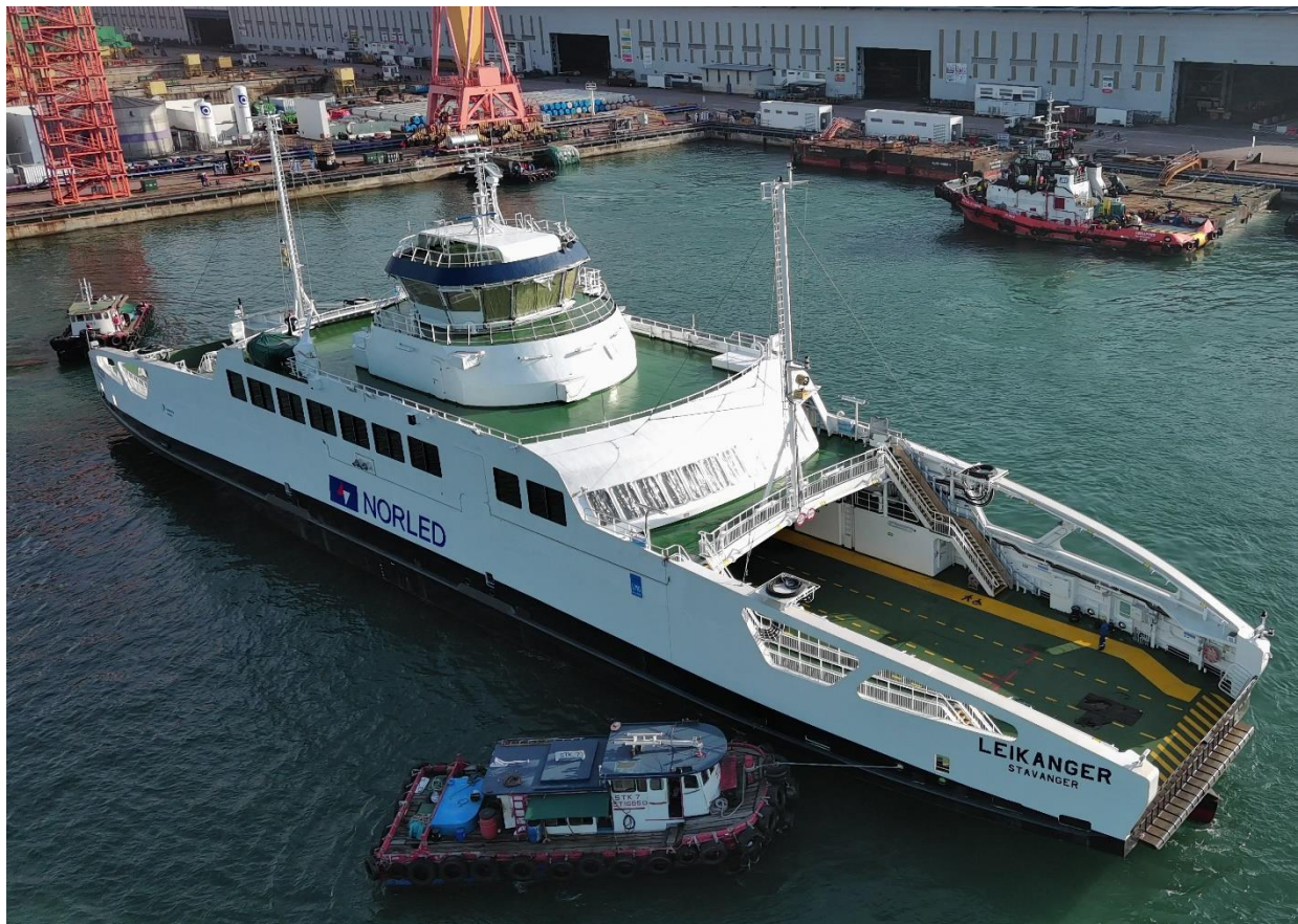
Leikanger – the final unit of three zero-emission battery-powered Ropax ferries constructed by Sembcorp Marine for Norled based on a proprietary design by wholly-owned subsidiary LMG Marin (Photo: SCM, all Rights reserved)
