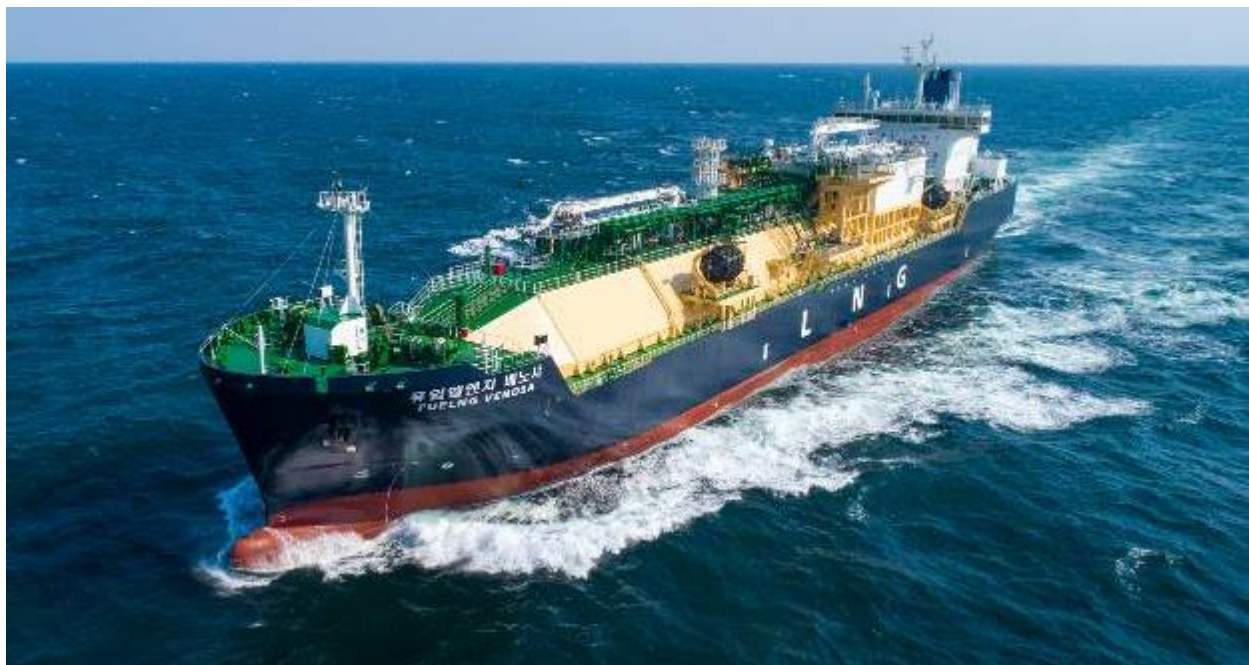
FueLNG Venosa, the latest state-of-the-art LNG bunker vessel to join FueLNG's fleet, is built for enhanced efficiency and performance, with a total capacity of 18,000 cbm (Photo: FueLNG, all rights reserved)
