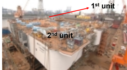
2 Upper Hulls of 2 semi-submersibles constructed simultaneously side-by-side
