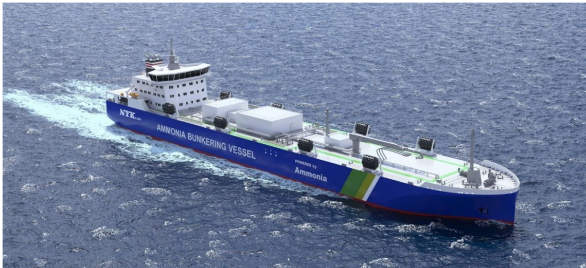
Illustration of the Ammonia-Fuelled Ammonia Bunkering Vessel (AF-ABV) designed by LMG Marin (a member of Seatrium Group). (Photo Credit: Seatrium Limited)
